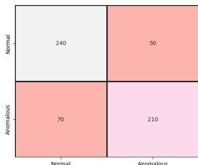
Fig.4. Confusion matrix for data error detection of the High-Speed Shaft Upwind Bearing Radial sensor.
