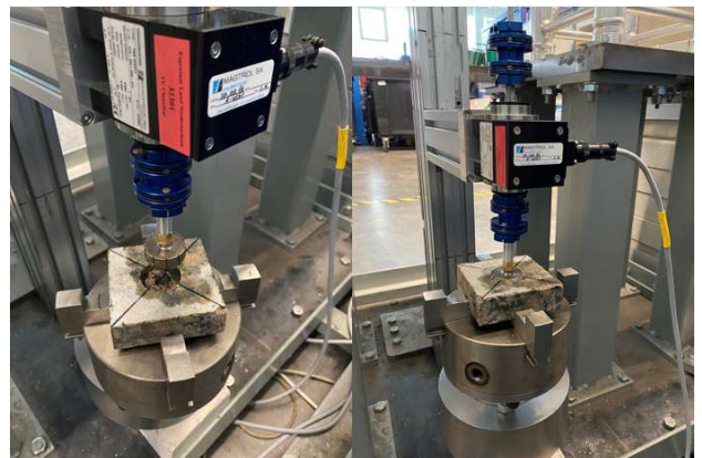
Fig. 4. Setup of the sample holder for clamping the rock samples.
