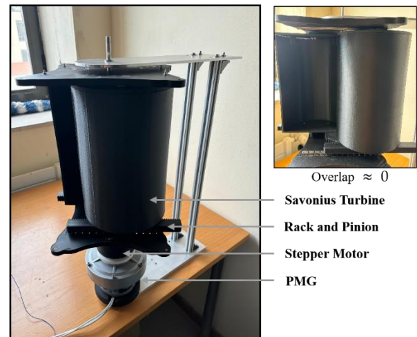
Figure 9 : Savonius turbine with pitch control
