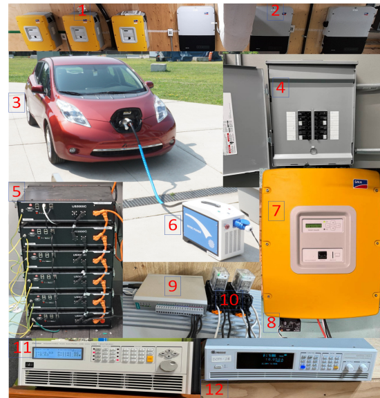
Fig. 9. Devices used in the proposed test bench: 1. Sunny Islands, 2. Sunny Boys, 3. Nissan Leaf, 4. Sub-Panel and Loadshedding Relays, 5. Pylontech Battery, 6. SETEC V2H Inverter, 7. Sunny Island 4, 8. EV to SI4 Relay, 9. ioLogik, 10. Interface relays, 11. Programmable Load, 12. PV Emulator.
