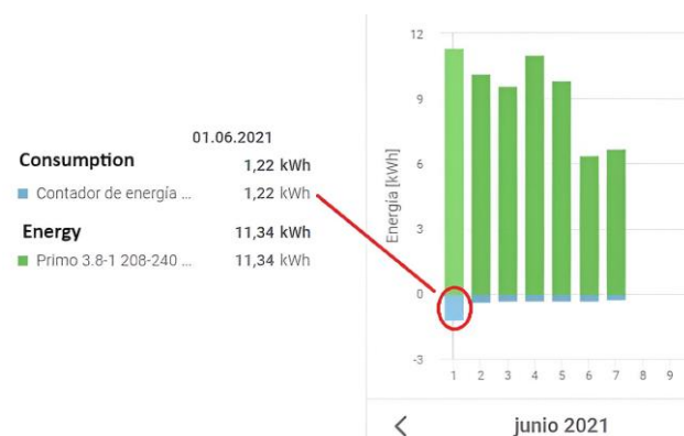
Fig. 12. Total PV generation and energy demanded by EV.
