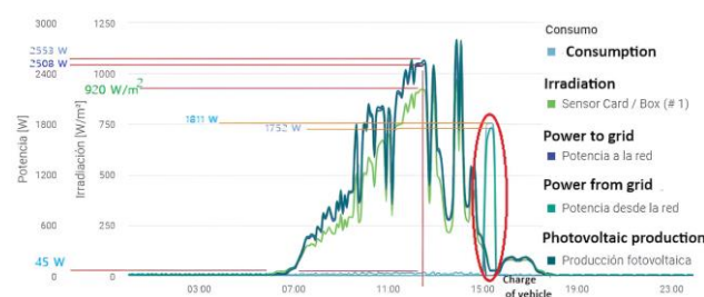
Fig. 10. Curves of relevant variables observed during the charging process of the electric vehicle.
