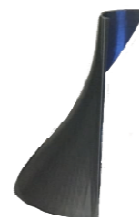
Fig. 3. Real-scale 3D printed blade model.
