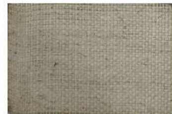
Fig. 1. Fique fiber laminate with unsaturated polyester resin
