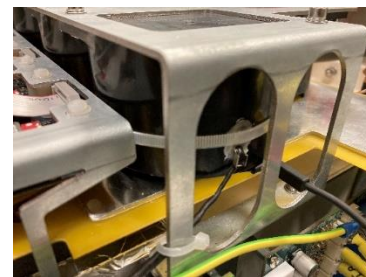
Fig. 7. Capacitor case temperature sensor arrangement
