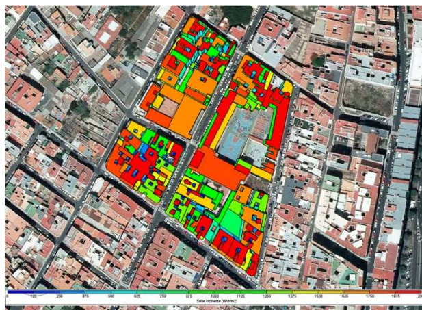
Fig.8. Aerial photo of the study area in El Toscal, with incident irradiation normalized by roof surface ( \text{kWh/m}^2 \cdot \text{year} ) with the Meteonorm corrected climate file.
