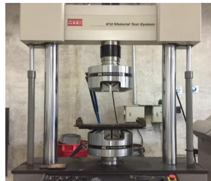
Fig.4. Flexotraction measuring equipment of the Universidad Industrial de Santander.
