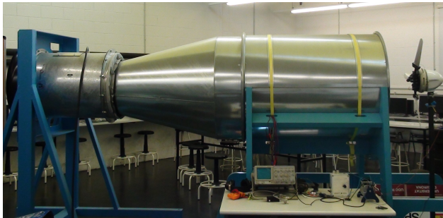
Fig. 1. Prototype installed at the exit of the open-circuit wind tunnel (right of the picture) ready to be tested.
